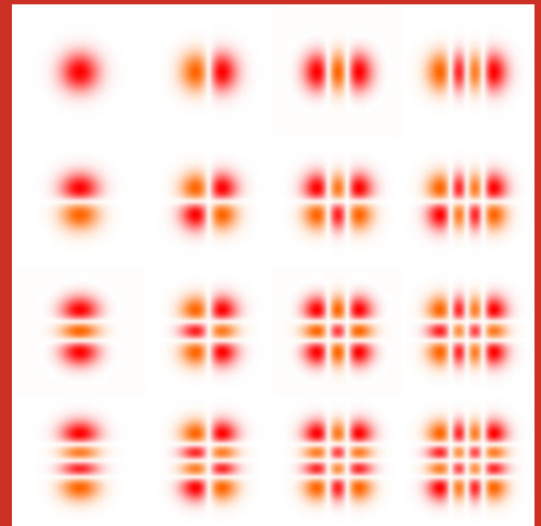
FIGURE 1: Hermite-Gaussian modes, starting from TEM 00 , m increases from left to right, n increases from top to bottom. Plotted is the the real part of the electric field at z = 0 . Red indicates a positive value for
